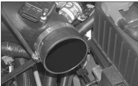
23. Secure the intake tube to the saddle bracket with the provided hose clamp as shown.
