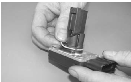
19. Remove the factory O ring from the mass air sensor as shown.
