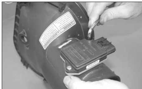
18. Remove the mass air sensor from the factory air box lid with the provided torx wrench as shown.
