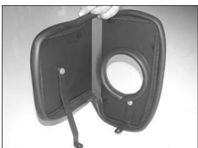
28. Install the two brackets onto the heat shield with the provided hardware as shown. Do not tighten completely.
