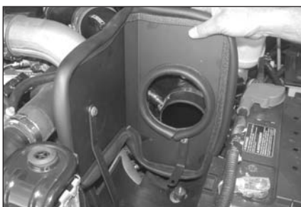
29. Install the heat shield assembly onto the vehicle as shown.
