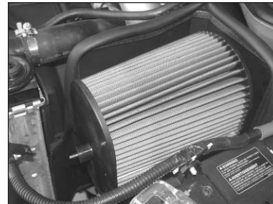
32. Install the filtercharger element onto the intake tube as shown. NOTE: Adjust all bracket and heat shield to obtain maximum clearance along the sides and under filter, then tighten the filter charger as shown.
