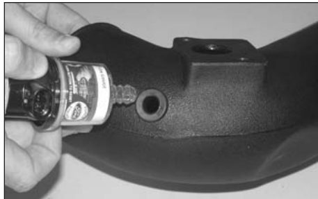
17. Install the factory grommet and restriction gauge onto the new K&N intake tube as shown.
