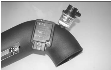
21. Install the mass air sensor onto the new K&N intake with the provided screws and spacers as shown.
