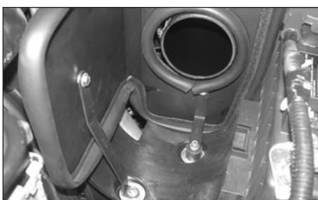
30. Mount the heat shield onto the rubber mounted stud and then secure the long "L" bracket onto the air box mount with the provided bolt and washers.
