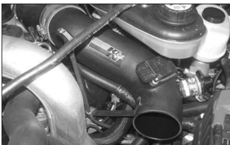
22. Install the new intake tube onto the turbo inlet with the provided hose clamp.
